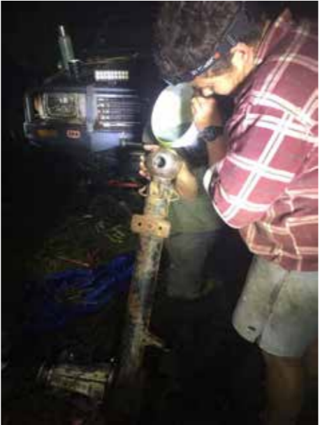
Refilling the rebuilt hi-lux axle with oil
